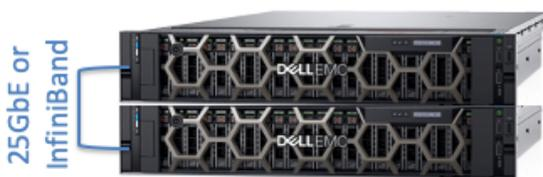
**FIGURE 1: Two Dell EMC PowerEdge R840 Servers configured as a 'couplet'**
